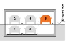
The vehicle on platform No. 5 can now be driven off the platform.
