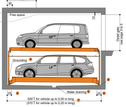
**PRODUCT DATA** trendvario 6100 2000 kg / 2600 kg / 3000 kg Individual parking spaces can even be loaded retrospectively! Loadable up to 3000 kg! Dimensions All space requirements are minimum
