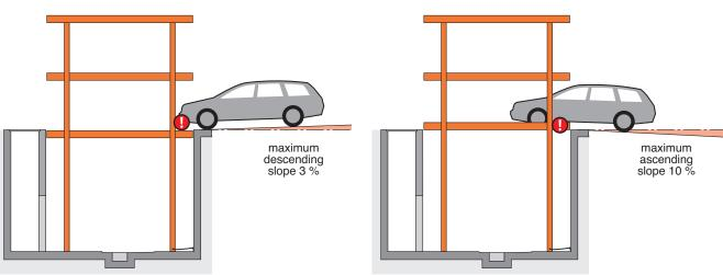
The illustrated maximum approach angles must not be exceeded. Incorrect approach angles will cause serious maneouvring & positioning problems on the parking system for which the local agency of KLAUS Multiparking accepts no responsibility.
