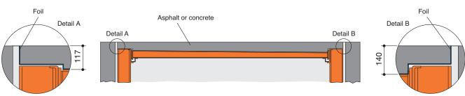
Before filling, the trough must be lined with a water-<u>im</u>permeable foil by a specialist company on site. Dimensions rounded.
