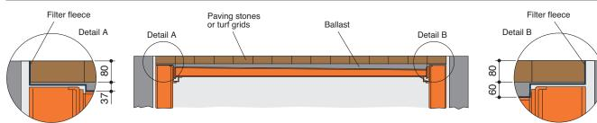
Before paving, the trough must be lined with a water-<u>permeable</u> filter fleece by a specialist company on site. Dimensions rounded.
