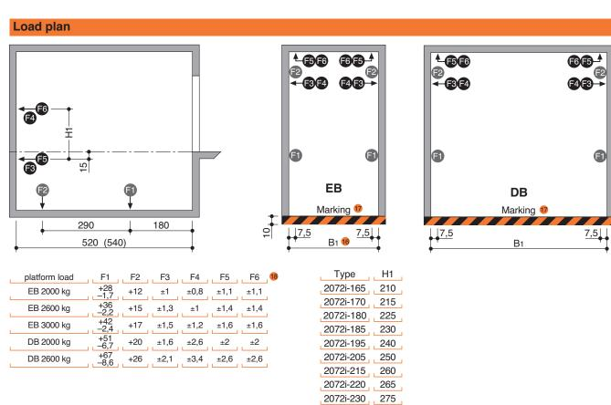
Units are dowelled to the floor. Drilling depth: approx. 15 cm.
