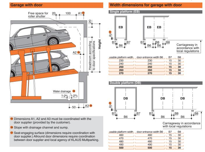
For parking boxes on the edges and boxes with intermediate walls we recommend our maximum platform width of 270 cm for single platforms and 500 for double platforms. Problems may occur if smaller platform widths are used (depending on car type, access and individual driving behaviour and capability).
